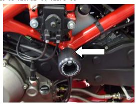
Please note that the way the kit is packed does not necessarily represent the way of mounting to the bike Please note that in cases where kits are packed with rubber washers holding the components onto the bolt – *the rubber washers should be thrown away*!
