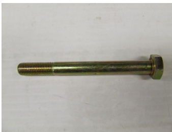
2 x M10 x 1.25 x 100 Hex Head Bolts FRONT PROTECTORS
